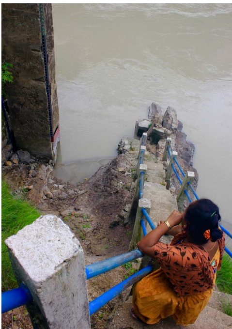
Fig. 6. Chisapani’s gauge reader observes the Karnali River’s water level using a manual gauge. Photo by author.
