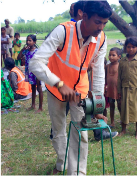
Fig. 1. An example of a hand-operated siren used within villages to alert and mobilize residents when an early warning is received. Photo by author.
